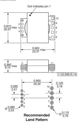
Note: Pad for pin 3 not necessary for schematics B, D and F. Pad for pin 8 is not necessary for schematics C and D. Pads 1 and 5 are only needed for optional auxiliary winding. Core material Ferrite
