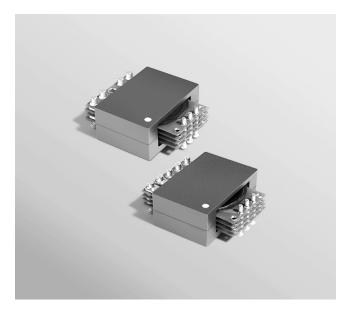
The PL140 surface mount planar transformers are rated for 140 Watts and are designed to operate between 200 kHz and 500 kHz. They are available in 15 turns ratios and six different schematics, and may be special ordered with an auxiliary winding.
