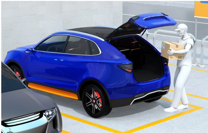
STO allows hands-free opening of the trunk with a simple kicking motion
